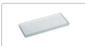
50mm reading scale (check magnification accuracy)
