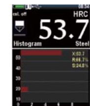
Histogram display mode, show average value, relative range and relative standard deviation
