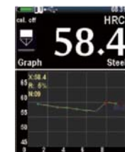
Graph display mode, show average value, relative range and test times
