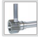
ultrasonic probe to test narrow areas (remove the cover)
