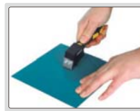
step 1: make grid cutting on surface
