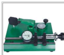
Inspect accuracy of dial indicators (range 0-25mm)
